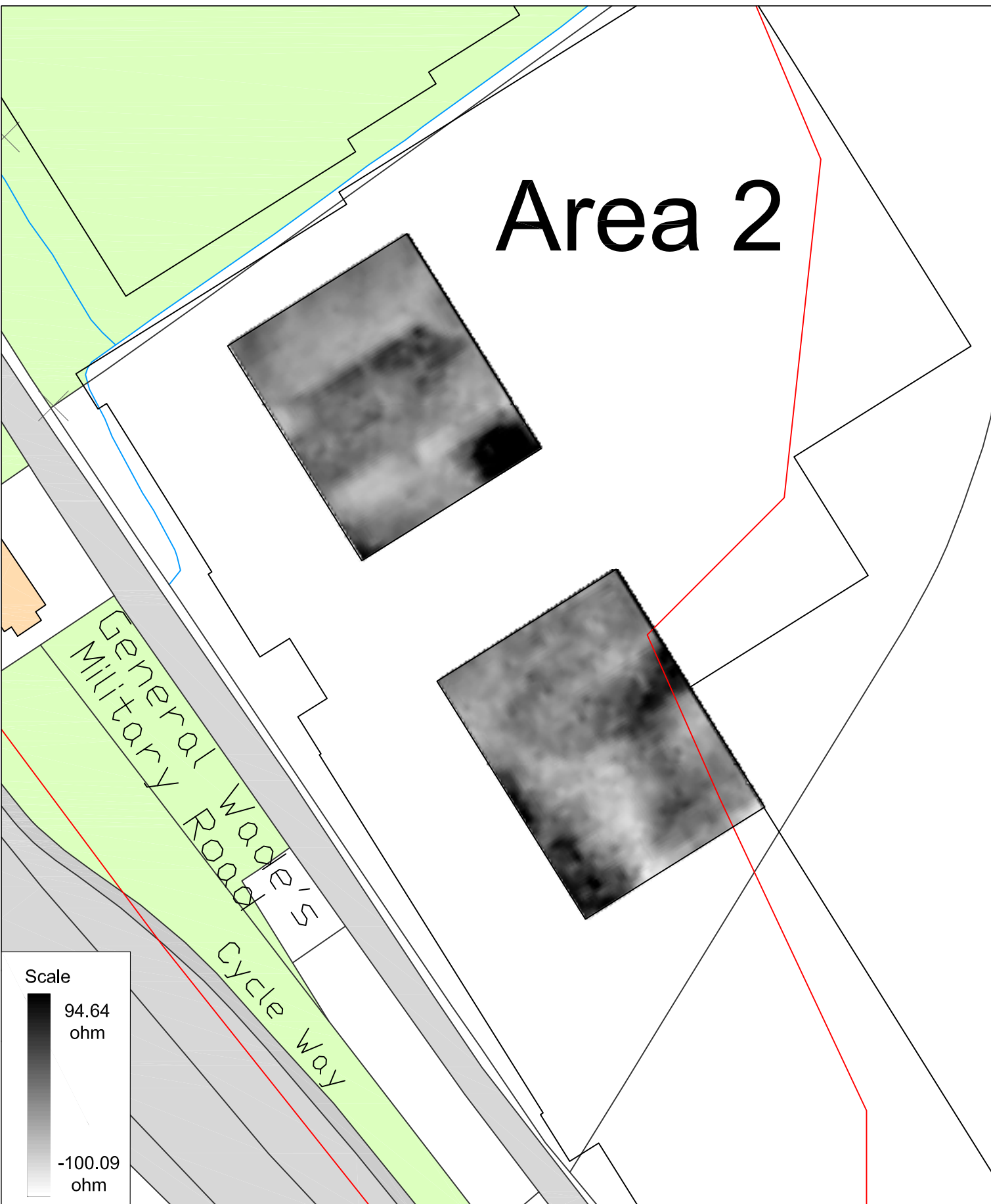
Processed earth resistance survey results - Greyscale plot - Dalmagarry
