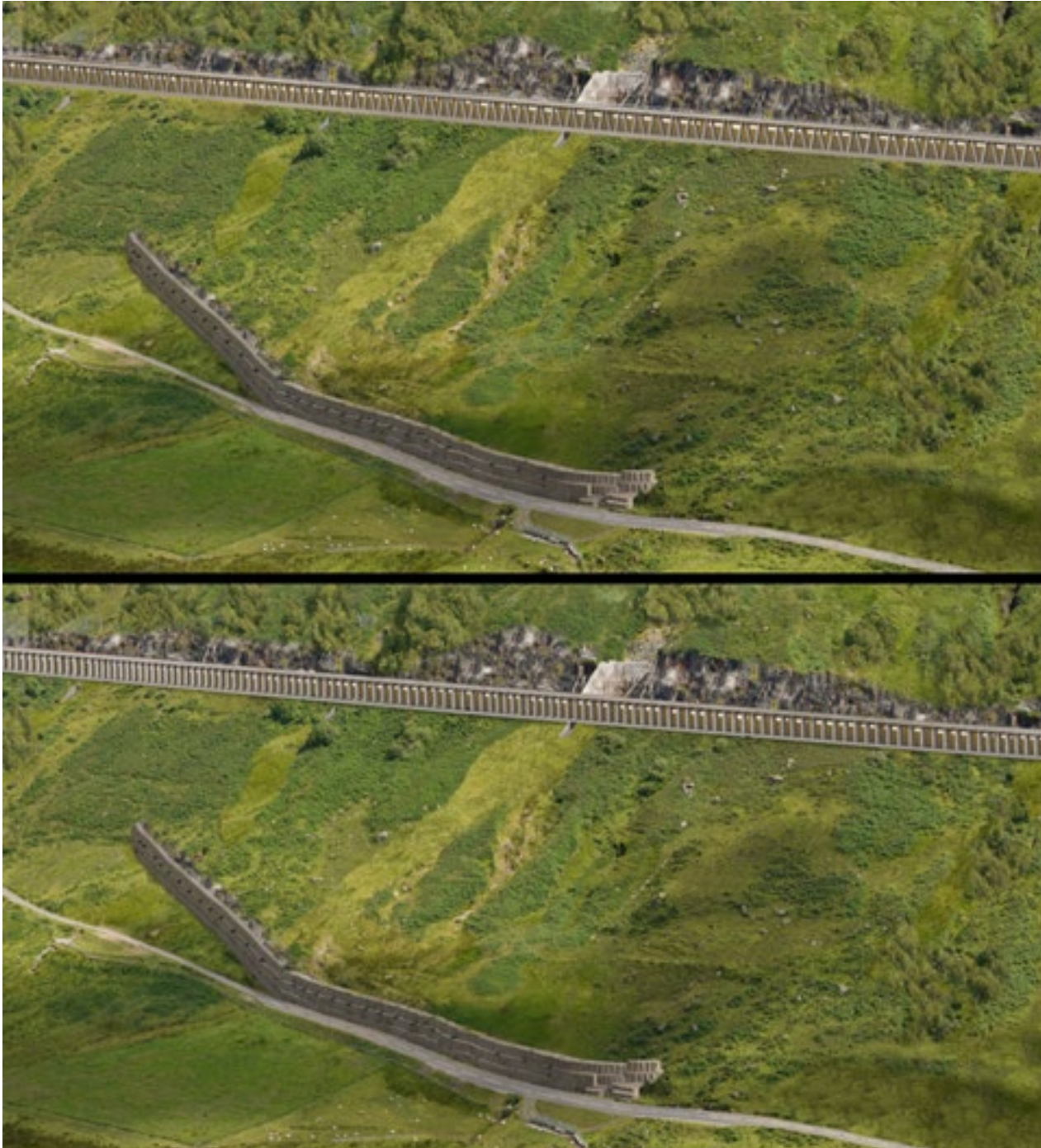
Figure 5 – Debris Flow Shelter (showing options for both vertical and slanted piers) and HESCO Barrier
