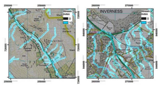
Figure 4.9 – Excerpts from the GIS showing the processed stream data as extracted from the Digital Terrain Model for two areas; (left) Glen Ogle and (right) Inverness. (OS Data © Crown Copyright. All rights reserved Scottish Government 100020540, 2008.)
