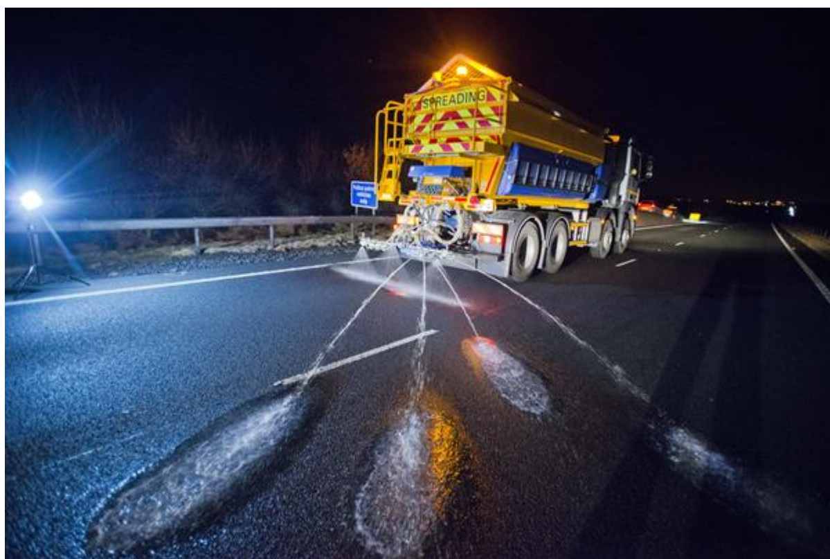
Figure 1. Brine spreading from the combi spreader
