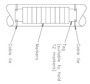
Typical Method of Marking Cables
