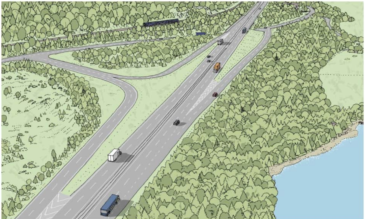
Illustration 12.3: Illustrative view of the proposed three arm junction at Birnam (Note that mitigation planting is indicative only and would be subject to further development)
