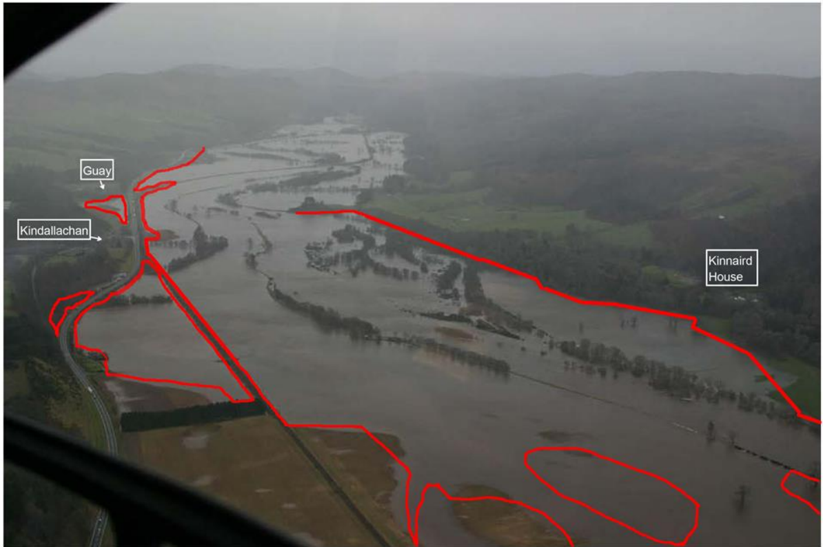
Diagram 17: Photograph of the December 2006 flood event, marked up with a sketch of the modelled flood extents for this event
