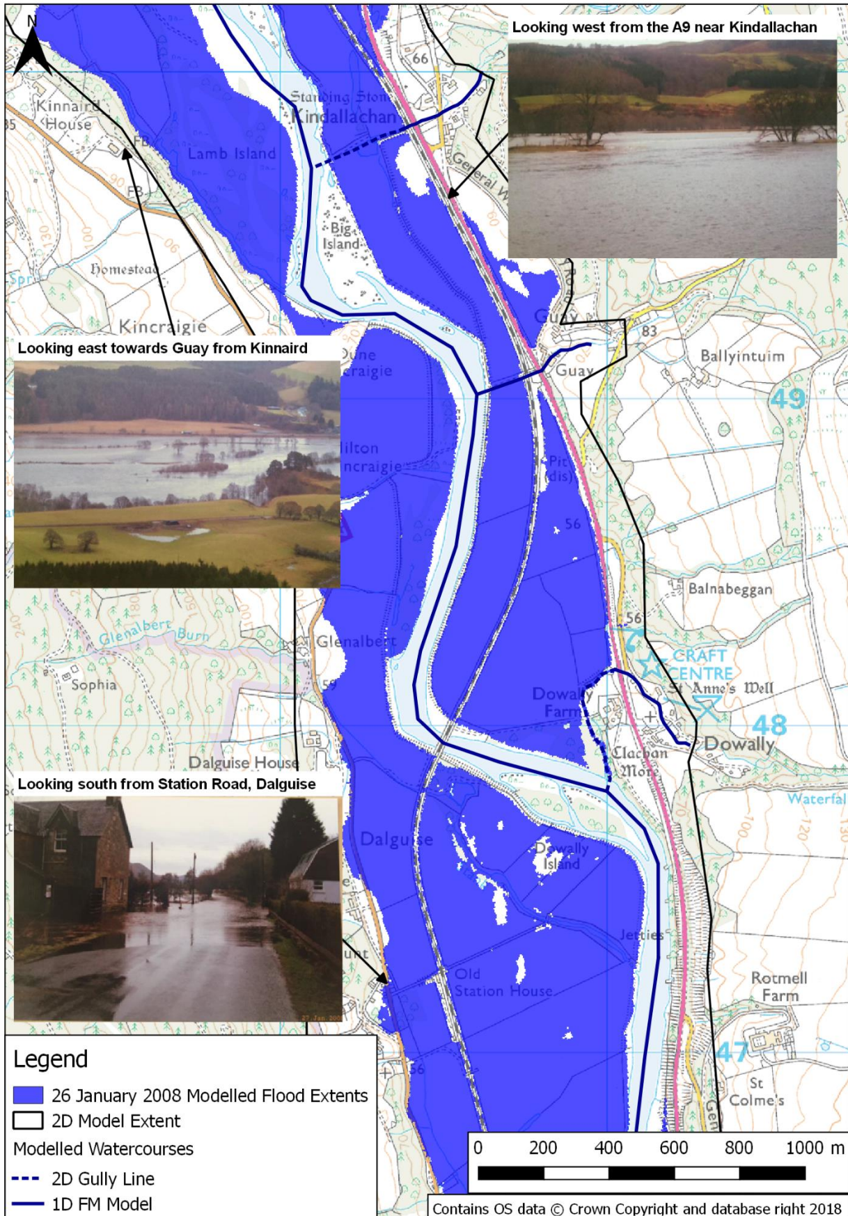
Diagram 16: Comparison of modelled flood extents with historic photos for the January 2008 flood event
