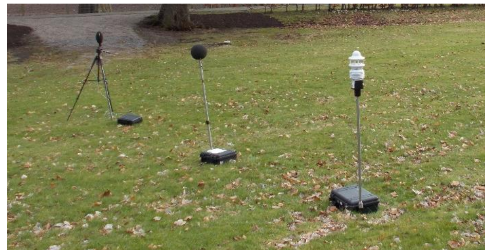
Photograph 9: Baseline noise monitoring equipment
