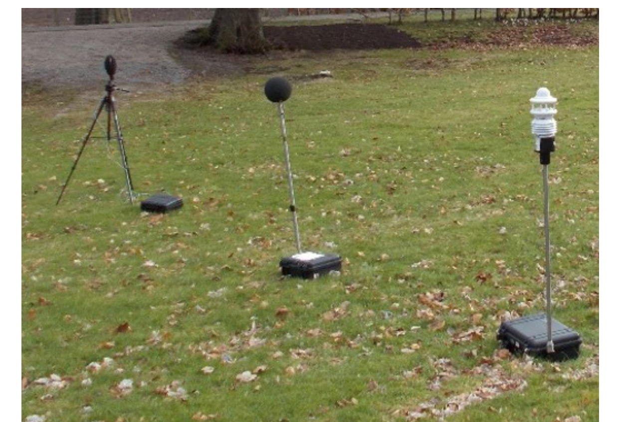
Baseline noise monitoring equipment
