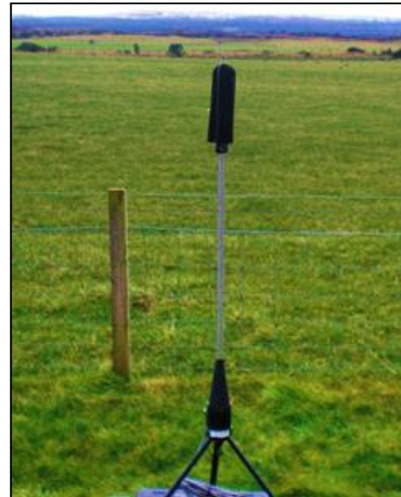
Photograph 2: Baseline noise monitoring equipment
