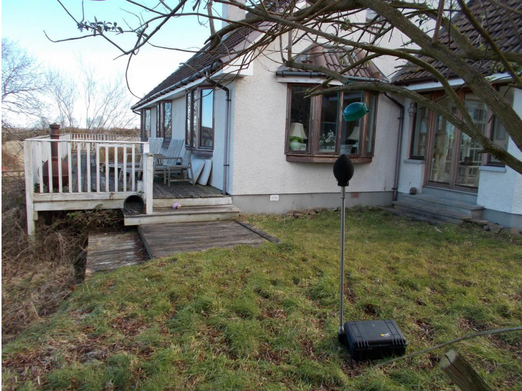
Photograph 5: Noise Monitoring Equipment at Annfield
