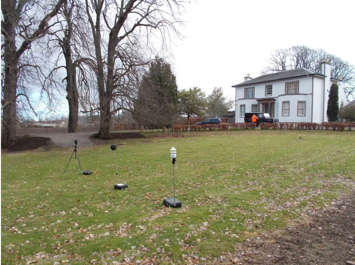
Photograph 2: Noise Monitoring Equipment at Castlehill
