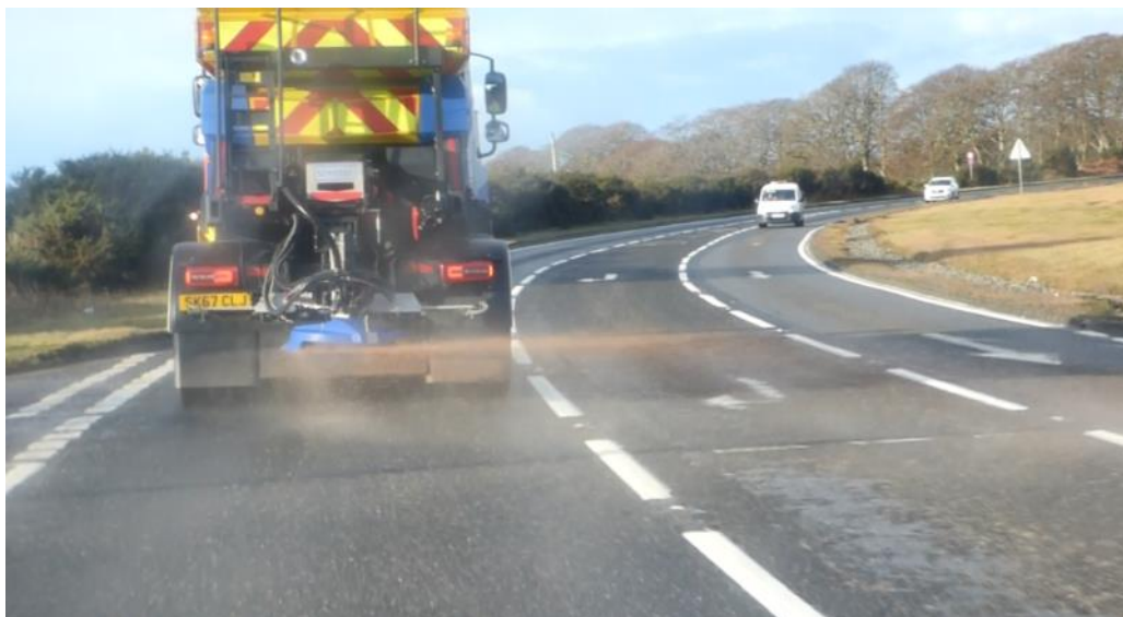
Figure 9. Spreading of pre-wetted salt required across junctions incorporating middle lane for right hand turning traffic.
