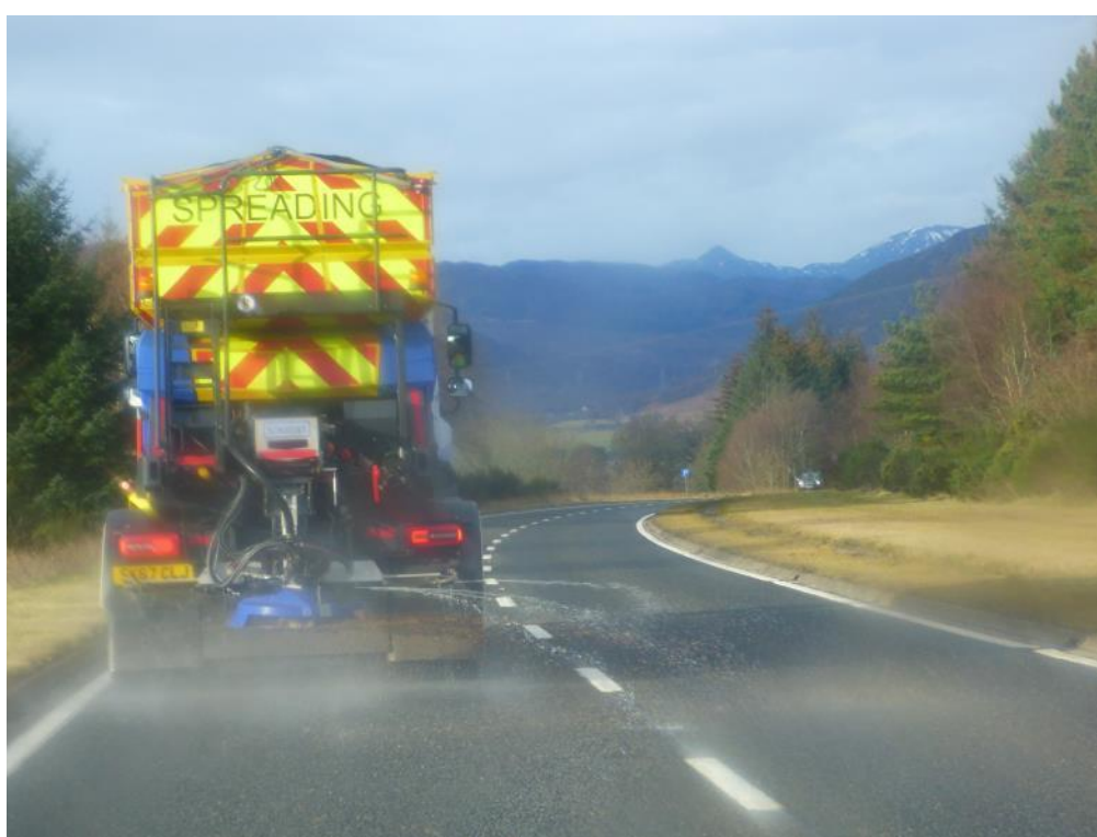
Figure 8. Brine spreading distribution in wind speeds approx. 5 – 10mph. Some deflection in brine jets visible.
