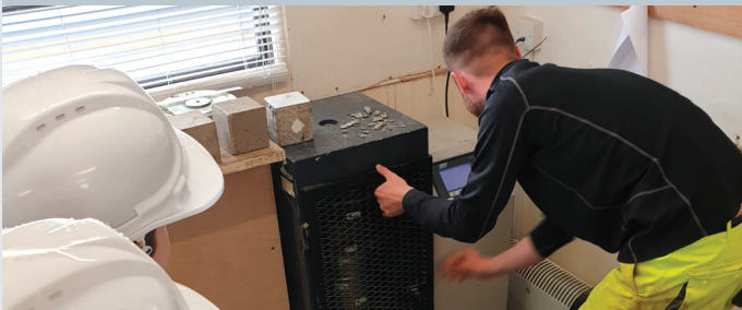
Concrete cube being crushed to destruction to test strength
