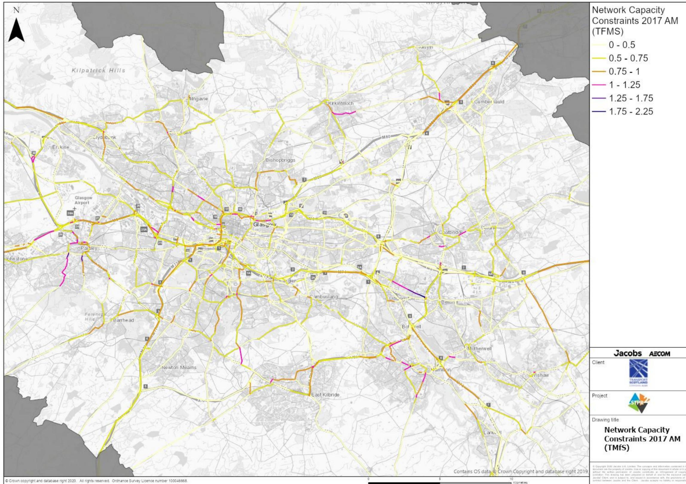
Figure A. 19: Network Capacity Constraints 2017 AM (TFMS) (click image to go back to main report)
