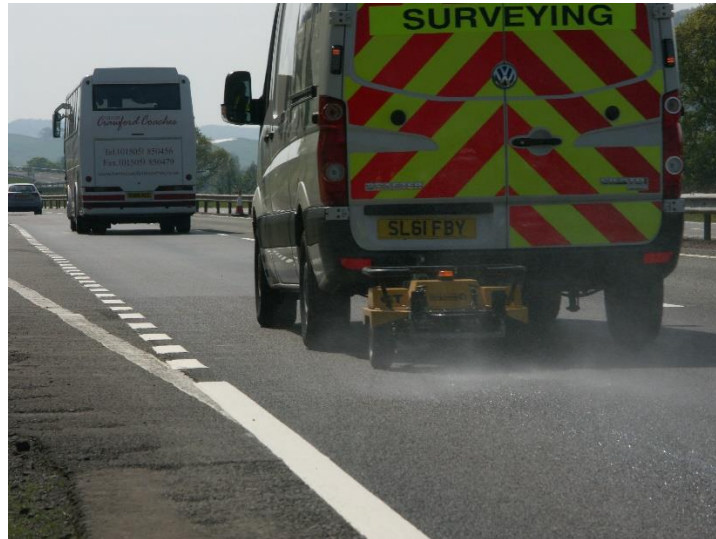
Figure 2-4 - GripTester measuring early-life skid resistance
