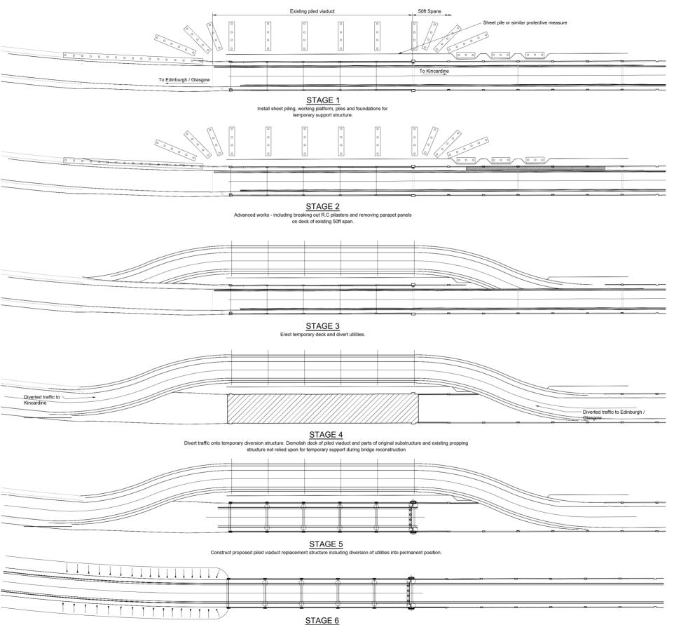
Divert traffic onto new structure. Remove and dismantle temporary deck. Remove temporary support structure and sheet piling, then cut piles down to 1m below ground level. Reconstruct R.C pilasters and parapet panels on 50tt concrete spans. Remove any remaining parts of original piled viaduct substructure and existing propping structure down to 1m below ground level
