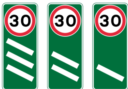
Figure 9: Countdown markers to the commencement of a speed limit
