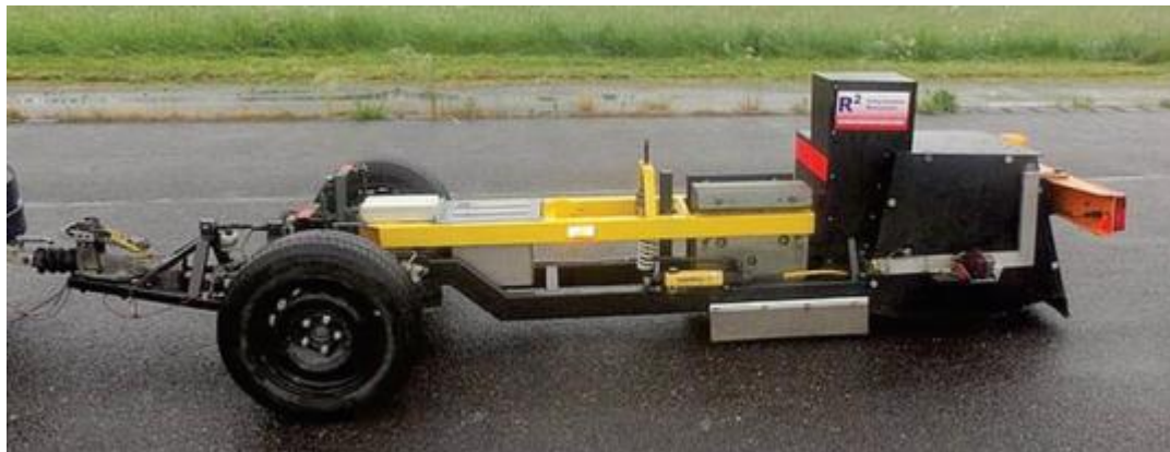
Figure 2-5 - TUG tyre/road rolling resistance measurement (Courtesy of Vejdirektoratet 8 )
