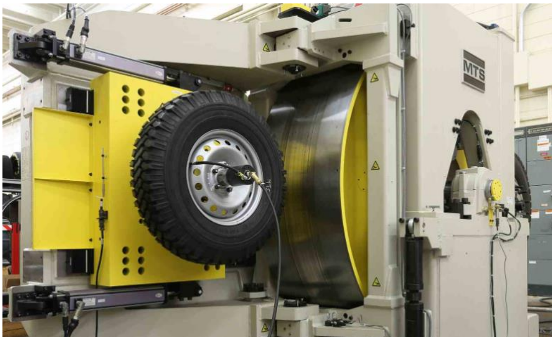
Figure 2-4 - Tyre rolling resistance system (Courtesy of MTS Systems)
