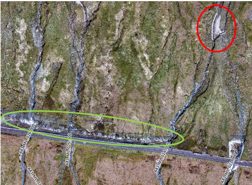
Plate A19.3.10 Upstream channel diversions (circled red) and large A83 catchpit into which multiple watercourses flow (circled green) (Aerial imagery: April 2024)
